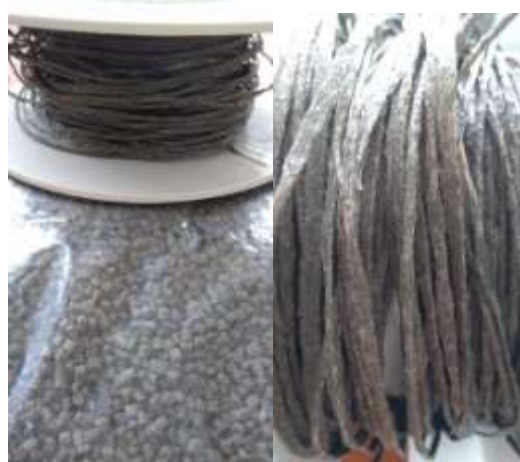
Figure 11 Produced filament from recycled HDPE with hay sawdust (ratio 90:10)
