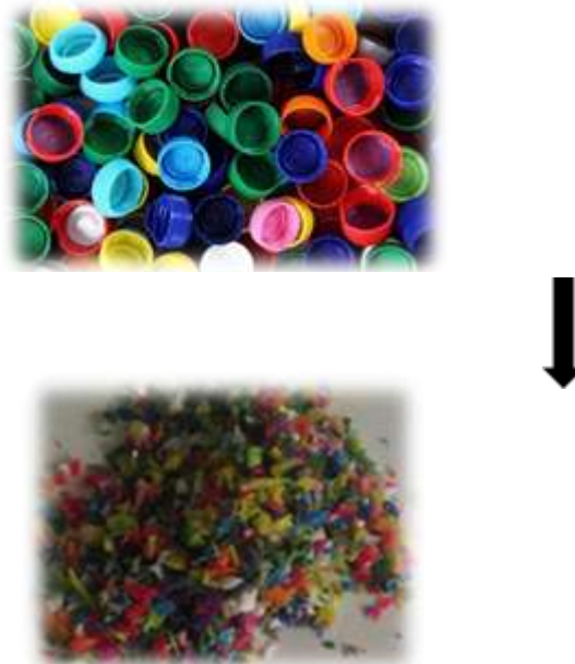
Figure 3 The disintegration of PET bottle lids
