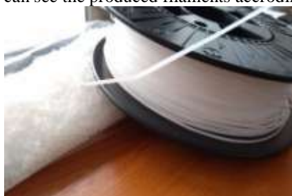
Figure 8 Produced filament from virgin HDPE
