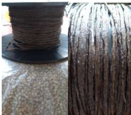
Figure 12 Produced filament from virgin HDPE with hay sawdust (ratio 80:20)
